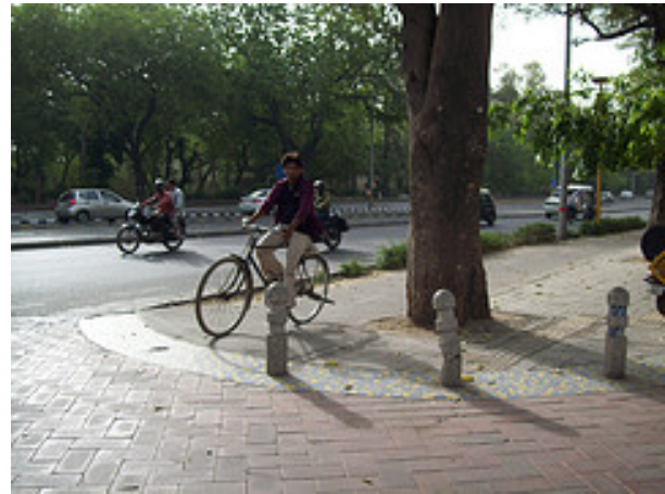
Illustration 5: Raised crossings and different materials enhance the safety of cyclists at intersections.
