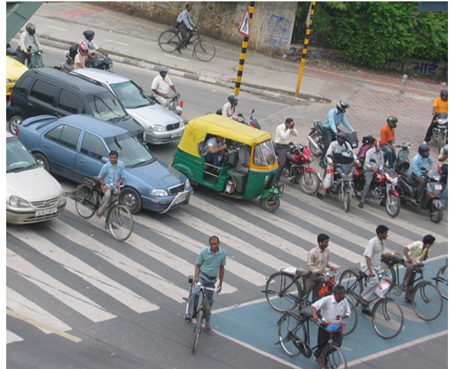
Illustration 7: Use of a bike box for cyclists turning right or going straight in Delhi
