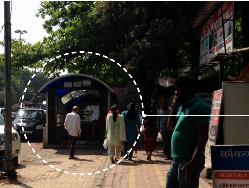
Entrance to subways bock either the footpath or the cycle track if there is not enough ROW.
