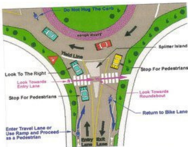
Fig. 31 Pedestrian Facilities at Roundabout
